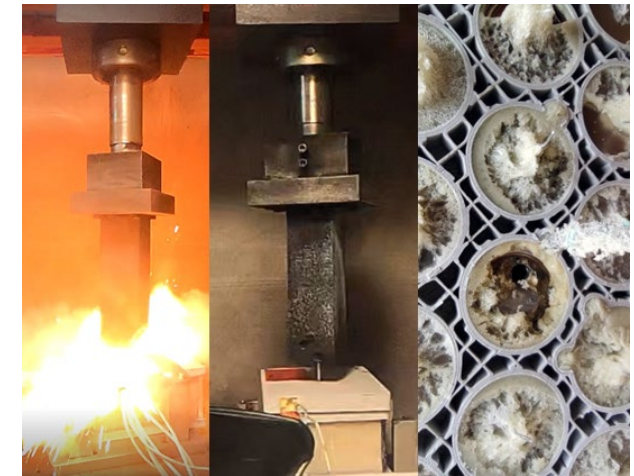
Figure 22. Typical Nail Penetration Test on Li-ion cell in a module causing TR with no foam (left). Nail Penetration Test with Full-Cell Encapsulation in PPR Foam (middle). TR fully contained with no fire and adjacent cells fully operational (right) © Xerotech Ltd.
