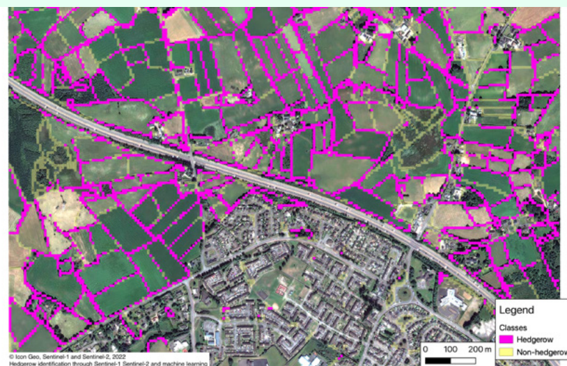
Figure 5. The image shows the Optical and Synthetic Aperture Radar (SAR) data sensed by the satellite and identification of hedgerows using AI-type processes © Icon Geo, Sentinel1 & Sentinel 2, 2022
