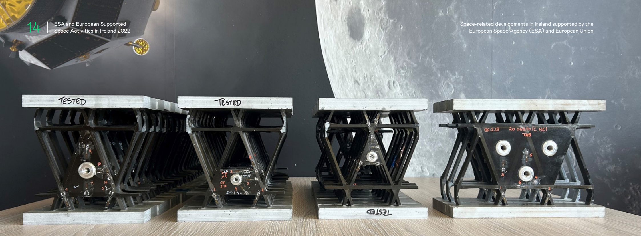
Figure 17. Integrated interface zones to be used in ATG Innovation's lattice satellite central tube structures. © ATG Innovation Ltd.
