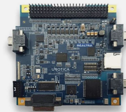
Figure 30: Réaltra Space Systems Engineering's RLT-AIA-001 AI Accelerator & Computer Vision Processing Board for CubeSats. © Réaltra Space Systems Engineering
