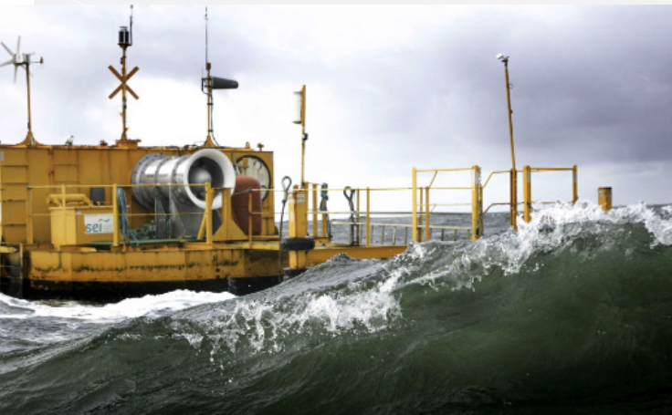
Figure 14: Ocean Energy's one-quarter-scale buoy undergoing sea trials. © Ocean Energy
