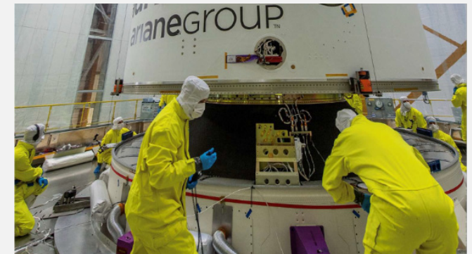
Figure 4: The VIKI hardware (developed by Réaltra Space Systems Engineering) is visible in the centre of this image of the James Webb Space telescope being encapsulated in the Ariane 5 fairing.
